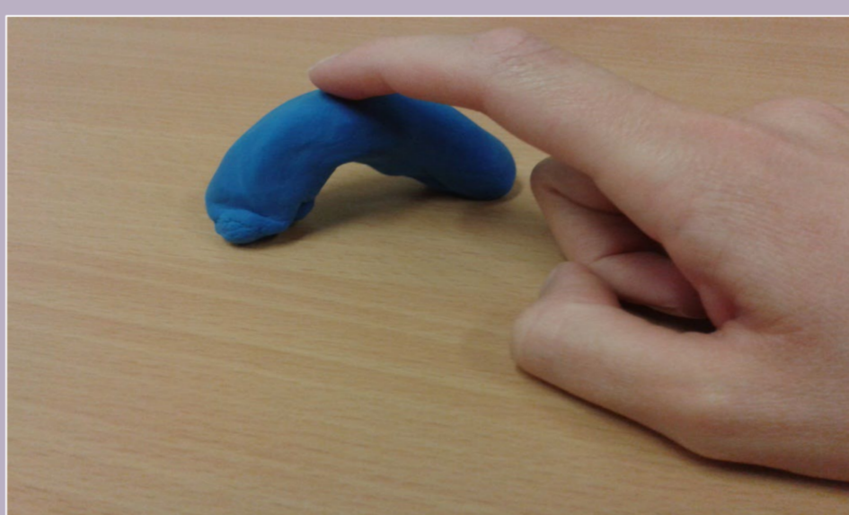
Fig. 3: Conductive modelling clay moulded to fit and connect with limited index finger movement in up and downwards motion
